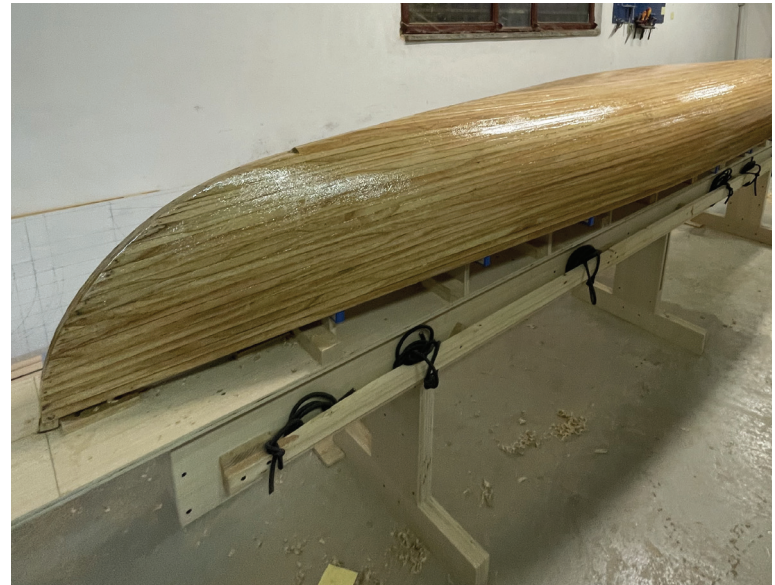
Top: The completed paulownia strip-planking on Gaia's latest build, before being sheathed in linen cloth and epoxy.
