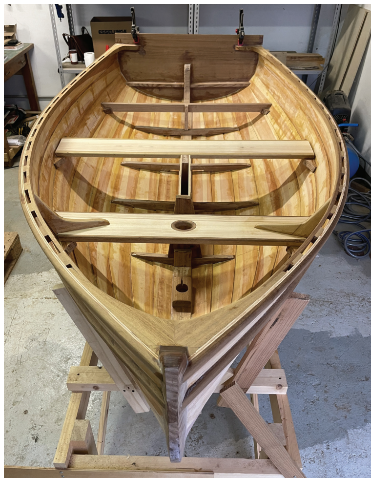
Facing page and above: Gaia's glued clinker build of an Iain Oughtred 7'10" (2.36m) Auk design, using Vendia marine plank. Left: Working to conserve traditional Italian boats in collaboration with the Vela Tradizionale association.
